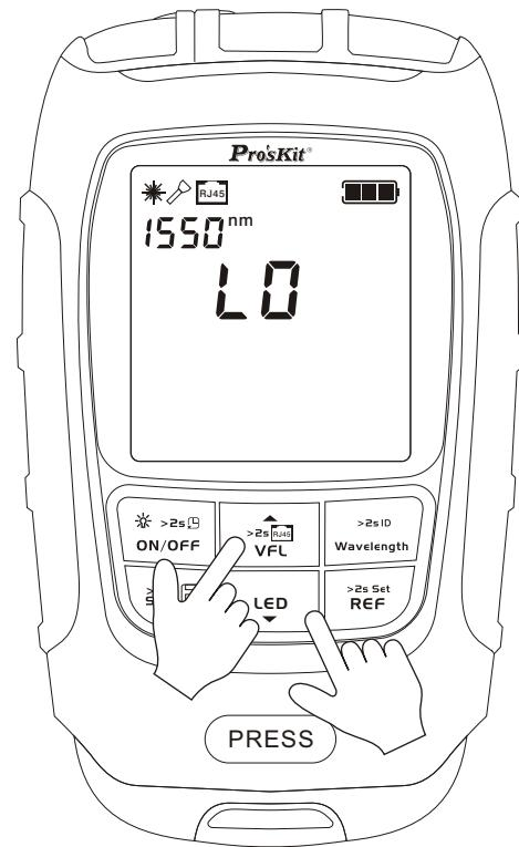
Short press "
