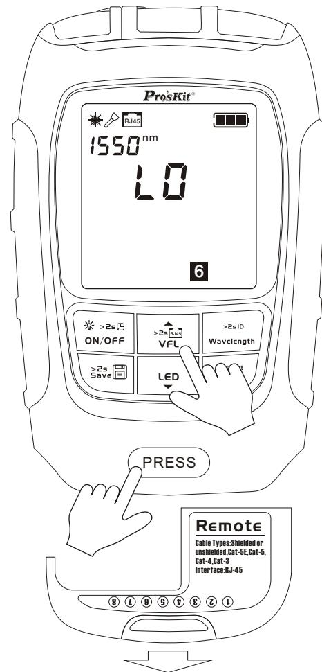
Press the module lock "press" key to pull out the module to test network cable , and push it back after testing;then make sure the module is locked tightly.Long press "
